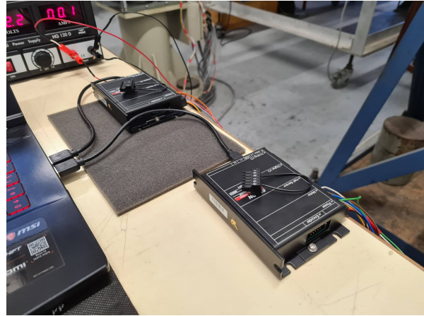
(b) ESCON 50/5 controllers close-up.
