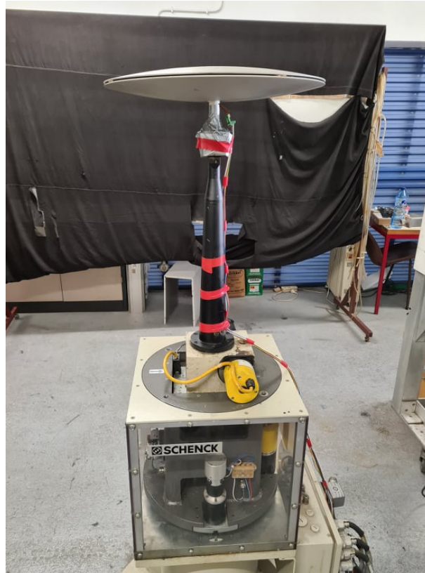
Figure 5.9: Aerodynamic scale assembly, the vertical support can be seen connecting the prototype (top) to the scale (bottom).
