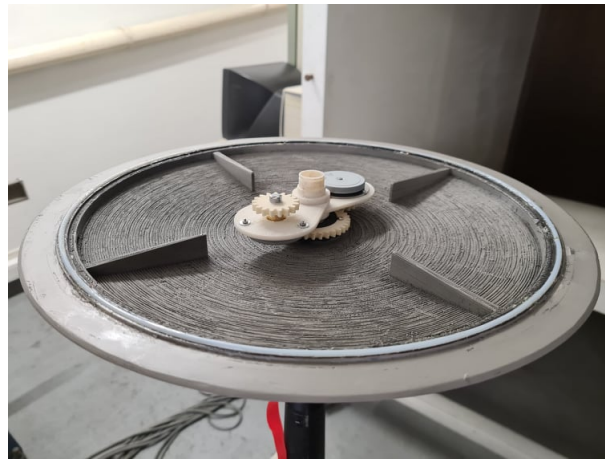
Figure 4.10: Prototype with bottom disc assembled (note the Teflon tube near the periphery).
