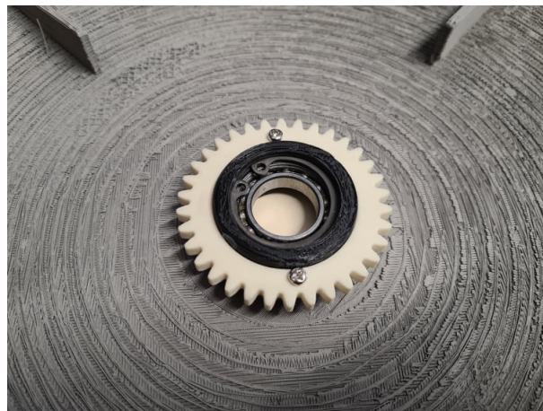
Figure 4.8: Top disc's casing with larger gear assembled.
